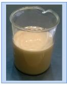
Pileman BH slurry, hydrated in fresh water is exposed to 10,000 ppm chloride hardness.
