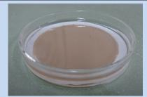
The 30% seawater diluted slurry is further used to form a filter cake and again exposed to sea water (35000 ppm total hardness). Under the effect of sea water, the filter cake remains to be stable.
