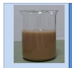
Diluted slurry with 30% seawater. No sedimentation.
