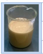
Pileman BH slurry, hydrated in fresh water is exposed to 10,000 ppm chloride hardness.
